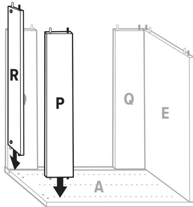
! The holes of part "P" must be towards the inside of the cabinet
